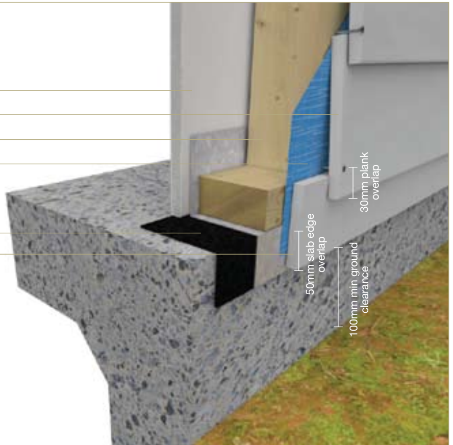
FIGURE 6A FASTENER DETAIL TIMBER FRAMING
